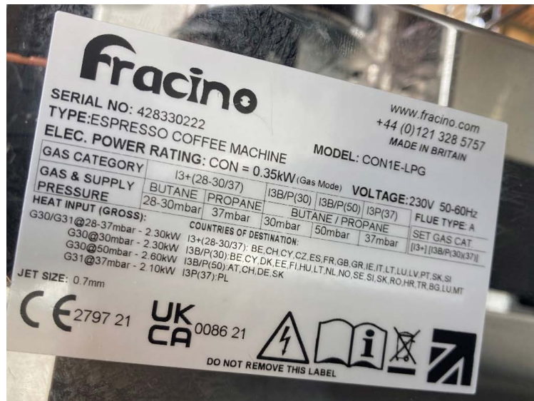
An example of an appliance data plate illustrating the conformity marking, manufacturers details, model details and power usage.
