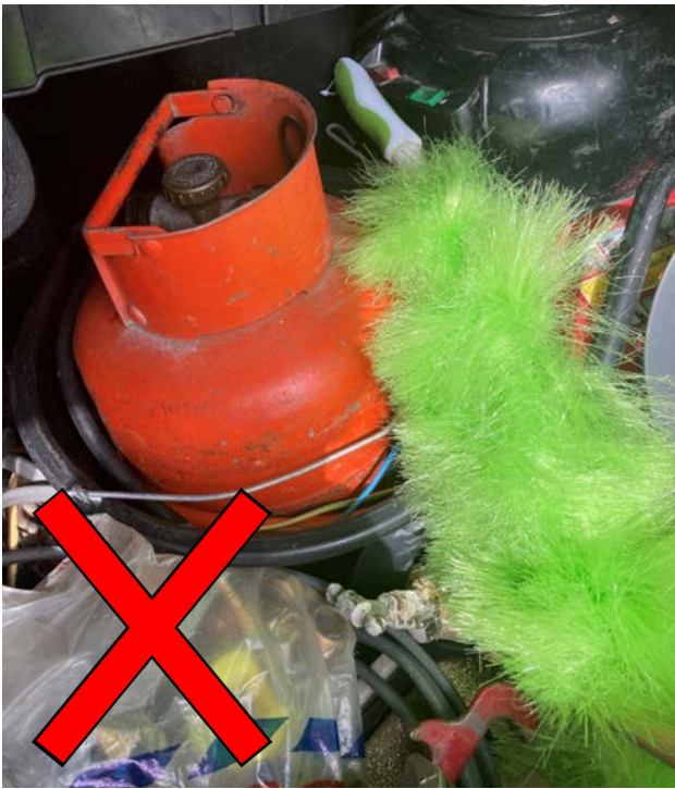
Incorrect transport - cylinder transported in the back of a van surrounded by an accumulation of combustible materials.
