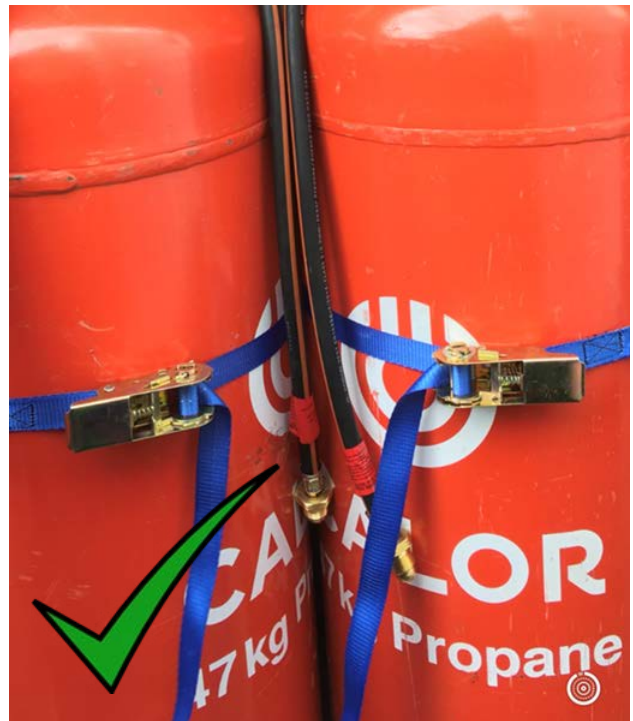
Cylinders transported inside a storage locker secured upright with suitable straps.
